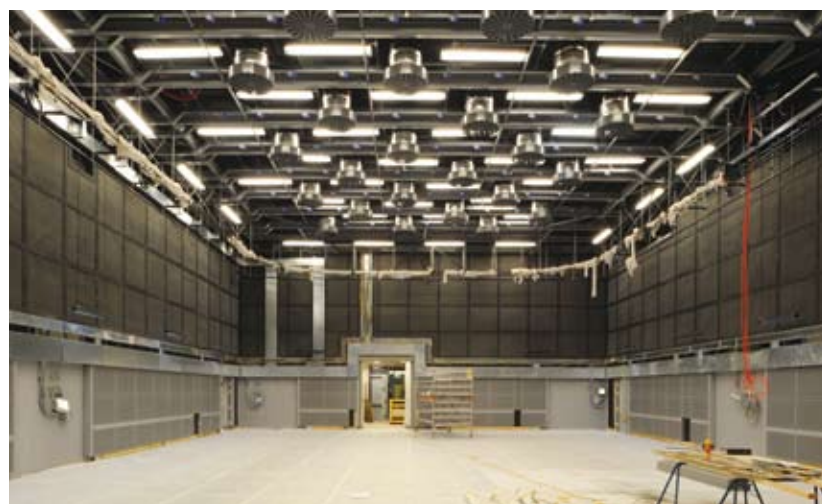
Television's flexible rig studio in the basement has the largest suspended floor in the world, designed to eliminate vibrations from underground trains
